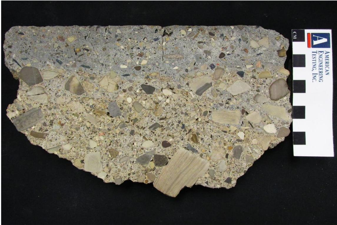
**Figure 3 – saw cut and lapped cross-sectional profile of Bellefontaine pavement sample. Note the two-layer construction is evident by both paste coloration and aggregate sizing**
