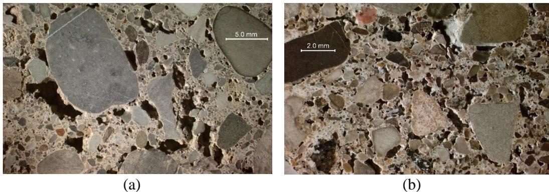
**Figure 5 – saw cut and lapped surfaces of the base concrete layer showing coarse irregular-shaped voids under 5x mag (a) and abundant voids producing a honeycomb' texture under 10x mag (b)**
