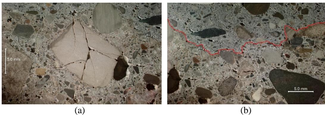
**Figure 11 – cracking within soft dolostone coarse aggregate particle within base layer concrete under 5x mag (a) and sub-horizontal cracking within base concrete paste near the contact with the wear-course (red line) under 5x mag (b)**
