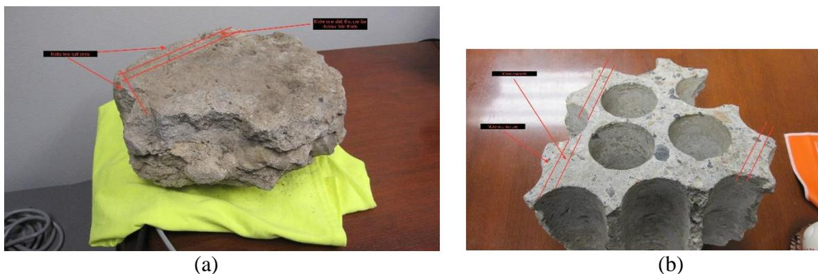
**Figure 2 – pre-submittal photos of intact concrete pavement segment (a) and previously-cored segment (b)** (photos supplied by the ACPA)
