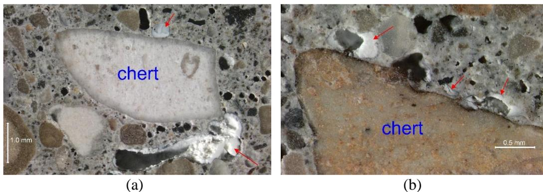
**Figure 12 – chert fine aggregate particles undergoing minor ASR within the wear-course concrete, red arrows indicate proximal deposits of secondary bright white ASR gel under 25x mag (a) and 50x mag (b)**
