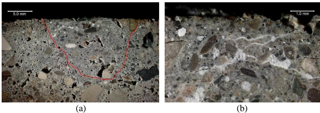
**Figure 10 – anomalous paste 'nodule' (red outline) near the pavement surface which lacks fine air voids under 5x mag (a) fine sub-horizontal microcracking within the nodule highlighted by white secondary deposits under 25x mag (b)**
