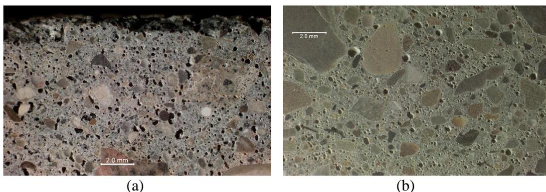
**Figure 6 – lapped section of top layer or wear-course concrete showing abundant (sub)spherical air voids within its paste under 10x mag (a) and comparison to a modern concrete with purposeful air entrainment under 10x mag (b)**
