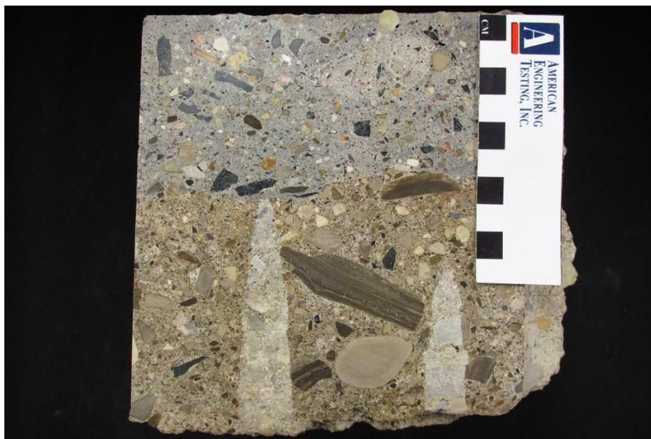
**Figure 9 – saw cut and lapped pavement section showing many dark and angular igneous rock particles within the wear-course topping, a few were also noted in the base layer.**
