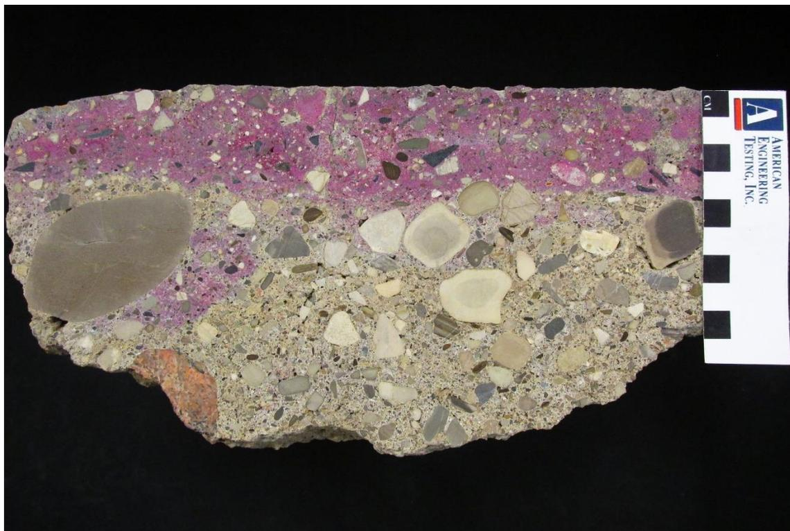
**Figure 4 – saw cut and lapped cross section of pavement after application of pH indicator. Magenta stain represents pH levels over 8.3. Note the base concrete exhibited lower pH associated with paste carbonation.**
