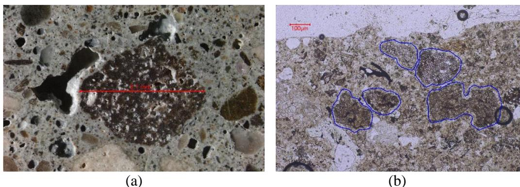
**Figure 7 – a very coarse dark-colored remnant clinker particle with a max. dimension of 3 mm in the wear-course concrete under 25x mag (a) and variable clinker morphology (blue outlines) as viewed in thin section of the wear-course under plane polarized light at 100x mag (b)**
