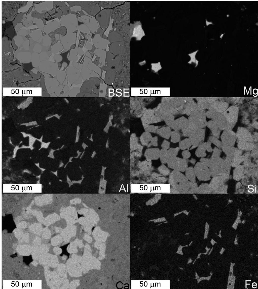
**Figure 8** – series of images consisting of a back-scattered electron (BSE) image (upper left) and subsequent elemental maps obtained from the same region. The element listed in the bottom right corner of the images denotes its presence as brightly-lit areas. Note the few brightly-lit areas in the Mg map which are attributed to the presence of magnesium oxide or periclase (MgO). Images from (Avdyllari, 2017).
